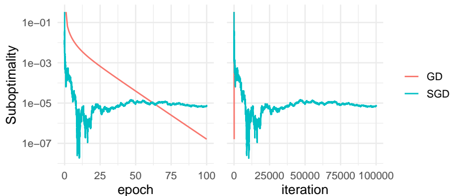
Figure 15: Convergence of gradient descent (GD) and stochastic gradient descent (SGD) for logistic regression in terms of iterations and epochs.
